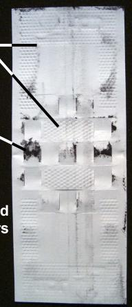
The product depicted here was used in the JCM UBA model. The JCM validator sensors, belts and rollers were dusted with a black chalk dust for this comparison photo. The Original Waffletechnology Cleaning Card was inserted first, then it was followed up with the new JCM Waffletechnology Cleaning Card. The results are dramatic! Use the right tool for the job...JCM Waffletechnology.
